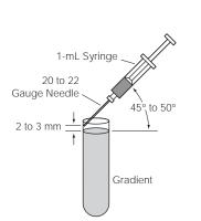
You can also prepare preformed step gradients by hand, using a pipette. Carefully layer solutions of decreasing concentration by placing the tip of the pipette at the angle formed by the tube wall and the meniscus, or float the lighter gradient concentrations up by adding increased density solutions to the tube bottom using a hypodermic syringe with a long needle such as a pipetting needle.
