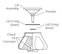
Frequent and thorough inspection is crucial to maintaining a rotor in good operating condition.
