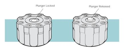
Figure 1-2. Plunger Mechanism in Locked and Released Positions (Vertical Tube Rotor Shown)
