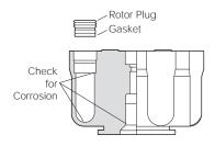
• Regularly check the condition of rotor plugs (a component of vertical tube and near vertical tube rotors) and rotor plug gaskets. Replace worn or damaged gaskets.
