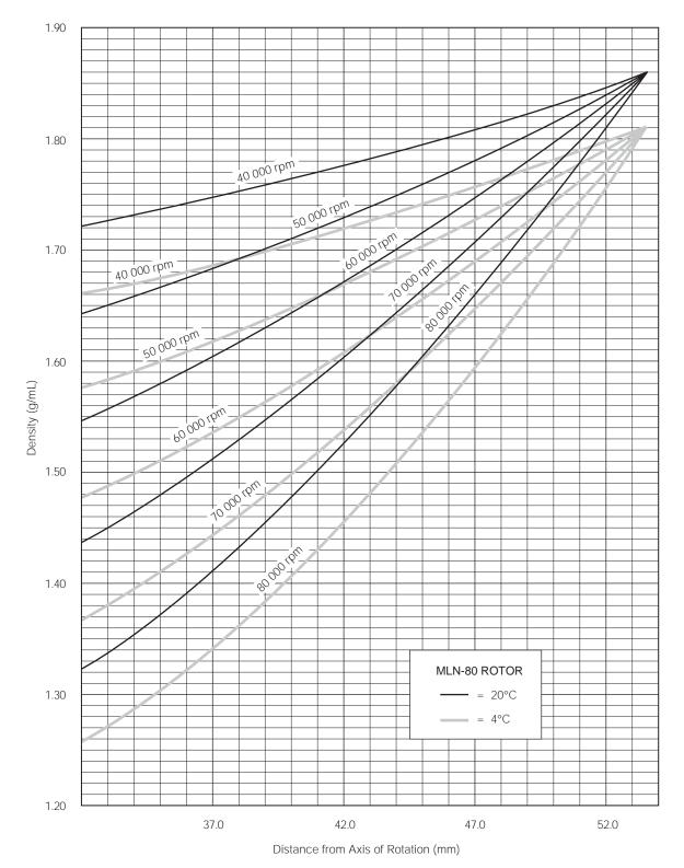
Figure B-2. CsCl Gradients at Equilibrium for the MLN-80 Rotor. Centrifugation of homogeneous CsCl solutions at the maximum allowable speeds
