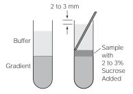
For *thinwall* tubes only partially filled with gradient, add a buffer solution to fill the tube to provide tube wall support. Although the gradient volume is reduced, sample volume is not changed.
