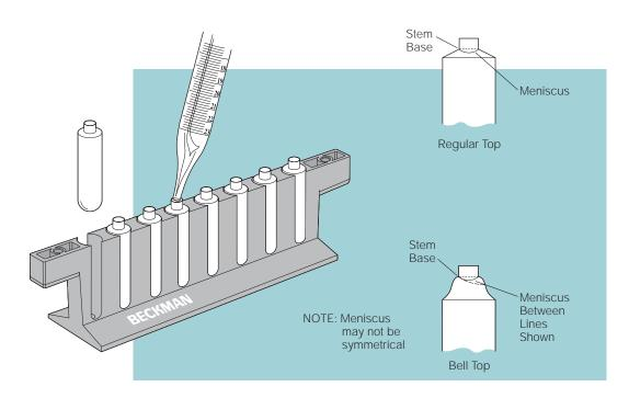
Figure 3-1. Filling OptiSeal Tubes. Stems are large enough to accept standard pipettes.
