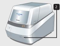
To start up the main unit without turning the heater ON, press and hold the sub-switch until a short beep is generated (for about 3 seconds).
